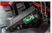
For the standard configuration, a less-angled accelerator pedal is provided to reduce the driver's fatigue.
